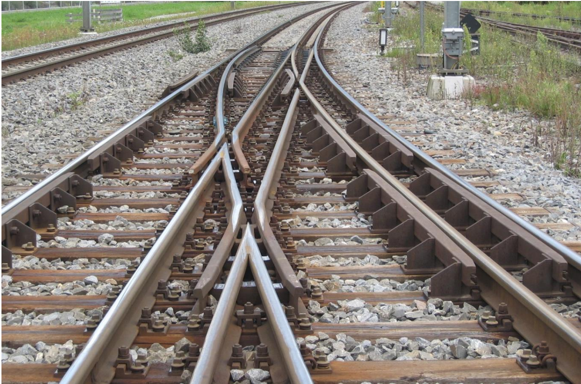
Switzerland „Felsberg“ T/O SBB I 185-1:7 type 4 1435/1003mm gauge
